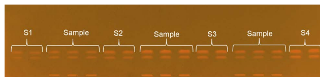
HPTLC chromatogram under UV 366 nm of wax esters in salmon samples spiked to contain 20 % wax esters ( n = 3 ) and standard solutions (S1–S4) of oleyl oleate ( hR_F 30) and stearyl stearate ( hR_F 40) after derivatization with Rhodamine B reagent
