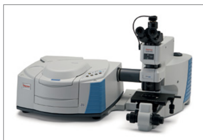
Figure 2: Nicolet iN5 with the Nicolet iS10 FTIR spectrometer.
