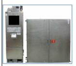
Having passed through the sample conditioning process the Hg is carried to the AFS detector. During the detection process, mercury is collected on a gold trap (amalgamation) which allows effective analyte concentration for total Hg whilst removing the sample matrix.
